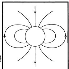
Schematic diagram of Earth's dipolar magnetic field, with lines and arrows showing orientation of magnetic field lines. The actual field tilts from Earth's spin axis. Because Earth's field is not a pure dipole, the north and south poles do not sit directly opposite each other.
