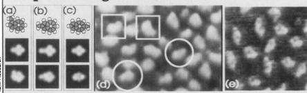
The scanning tunneling microscope's (STM) needle-like probe enables researchers to image the electron clouds surrounding atoms. Making sense of those images, however, requires detailed calculations that predict the shape of electron clouds for individual atoms. The task is even more difficult for molecules.
