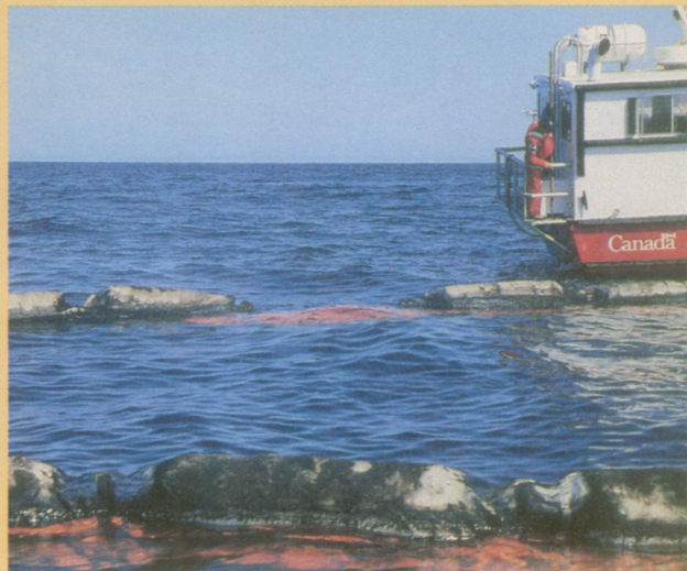
Photo shows missing float — one of the buoyant cylinders that anchors the boom's oil-containing skirt at water surface. This boom lost two floats from an experimentally redesigned segment.
