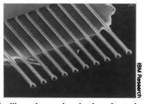
The aluminum-coated silicon levers bend when heated because these two materials expand by different amounts. The change in position shows how much heat has been absorbed, much as mercury expansion in a thermometer does. Lasers or measurements of changing electrical resistance detect how far the levers have bent, says Christoph E. Gerber, who developed the sensor at the IBM Research Laboratory in Zurich.
