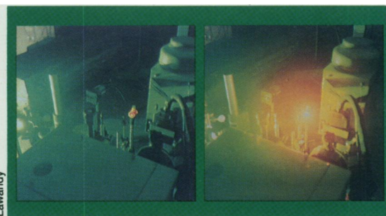
A green laser pulse excites a pure dye dissolved in a liquid to make the solution light up (left). A laser pulse of equal intensity sent into the same dye mixed with tiny particles of titanium dioxide suspended in a liquid produces a much stronger, room-filling glow (right).
