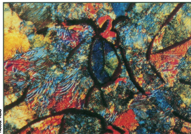
“The Web” (1971) shows the polished and etched surface of a gray iron casting taken from an automobile engine block. When magnified 800 times and viewed with reflected polarized light, layers of ferrite and a darker cementite give rise to colors.
