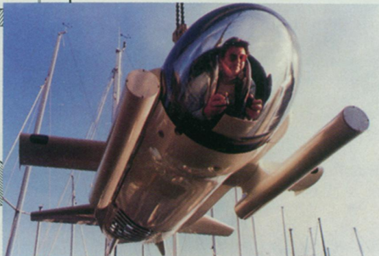
Diagram: Manipulating the wings, the pilot can counteract positive buoyancy and "fly" the submersible into the ocean depths. Photo: Deep Flight designer Graham Hawkes demonstrates the pilot's prone position.
