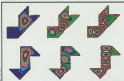
These images show the wave patterns observed experimentally in pairs of microwave cavities having different shapes but identical normal modes.
