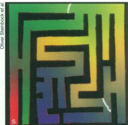
Computer map of optimal distances made by combining 250 images of a chemical wave that began at S. The farthest points are blue; white lines mark equidistant paths.
