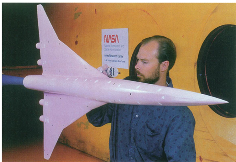
A n engineer makes a measurement on a model of an experimental supersonic transport. The model is coated with pressure-sensitive paint, giving its surface a pink color.
