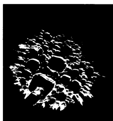
Stretching a drop of adhesive between two plates (top) creates voids within the drop, and fingers and cavities along its perimeter (right).
