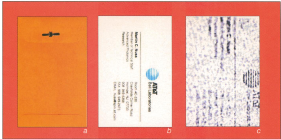
T rays pass through a sealed envelope (a), revealing an enclosed business card (b) and generating an image of the card (c).
