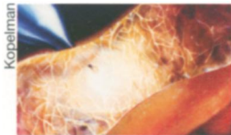
A fiber optic probe pierces a cell.
