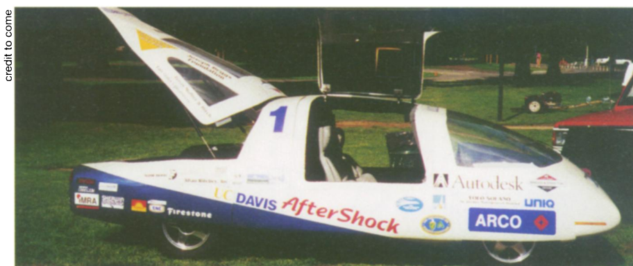
Fiberglass and other composite materials form the lightweight body of AfterShock, a two-seater hybrid electric vehicle built at the University of California, Davis. AfterShock can travel 500 miles on less than 6 gallons of gas, and its battery pack recharges in 6 hours—at a cost of 80 cents.
