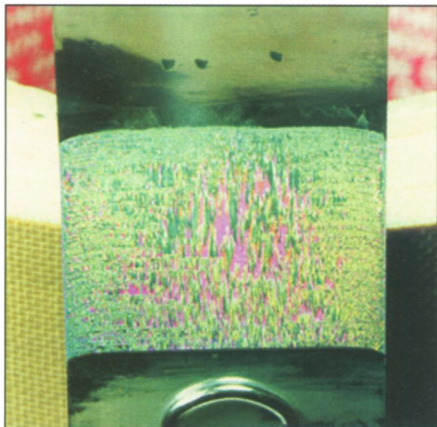
Glass slide coated with a layer of polystyrene particles. The slide is 2.6 centimeters wide, and the particles have a diameter of 953 nanometers.
