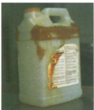
Orange stains illustrate extensive pesticide (trifluralin) penetration of HDPE container.
