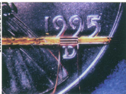
The size of the NMR microcoil in relation to a penny.
