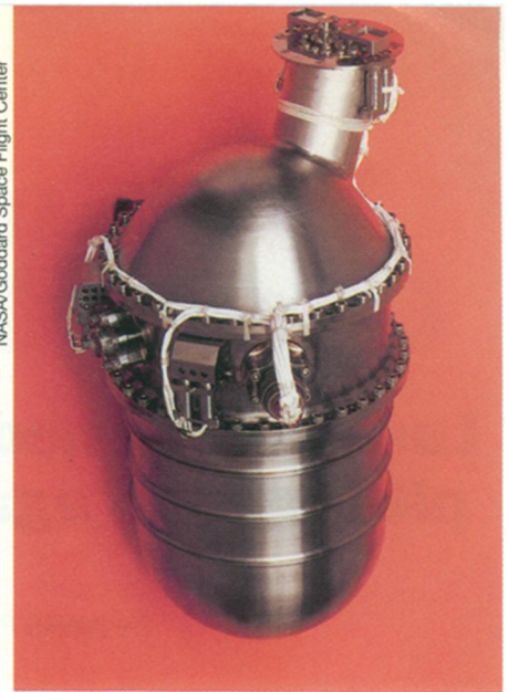
Duplicate of mass spectrometer, 0.4 meter tall, that plunged into Jupiter last December.
