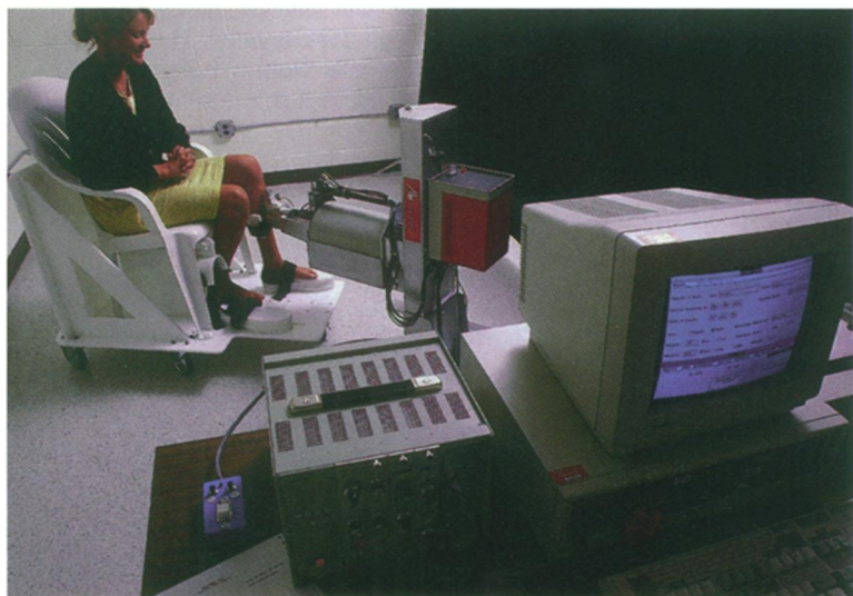
The KXRF instrument tests a woman's bone for lead concentrations.
