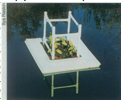
A floating garden of sunflowers absorbs radionuclides from a small pond on the Chernobyl site.
