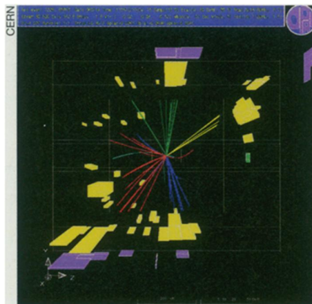
A computer display from the LEP collider Opal detector shows the result of an electron-positron collision. The interaction created a pair of W particles, both of which immediately changed into quark-antiquark pairs. The four quarks, in turn, transformed into four jets of detectable particles (tracks shown in red, yellow, blue, and green). Pink and yellow patches record the active detector sections.
