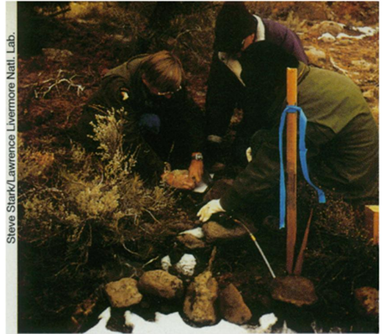
Lawrence Livermore scientists draw gas from a sample tube inserted in a fissure at the Nevada Test Site.
