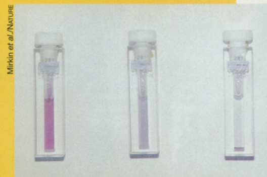
DNA-modified gold suspensions at 80°C (left) change color when they aggregate at room temperature (center), and precipitate out of the solution after several hours (right).
