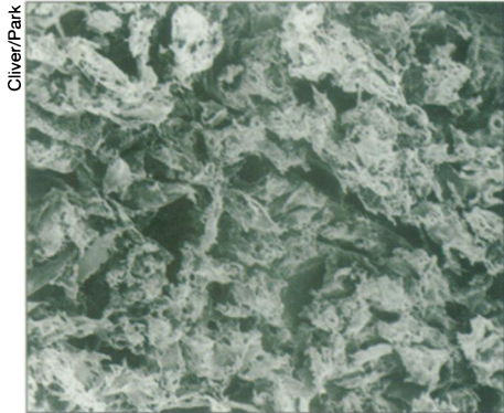
The surface of a knife-scarred plastic cutting board, magnified 36 times, shows niches where germs can hide.
