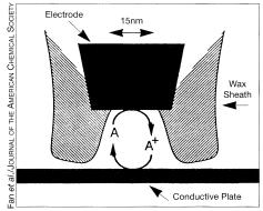
The single-molecule detection system. A wax sheath surrounds the tip of an electrode and, when lowered onto a conductive plate, seals off a small volume of solution. The volume contains a single molecule (A) of an iron compound; the molecule repeatedly gives up an electron to the electrode (becoming A+) and picks up one from the plate, thus producing a tiny, but measurable, current.
