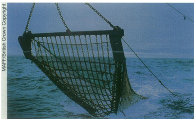
This 4-meter-wide beam trawl has a chain matrix to keep rocks and rough terrain from damaging the gear.
