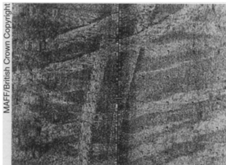
Sidescan sonar image from Irish Sea depicts marks scored on seabed by passes of a 4-meter beam trawl.
