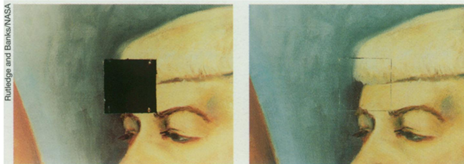
After exposure to smoke from an oil fire, a section cut out of a 15-year-old oil painting is covered with black soot (left). Treatment with atomic oxygen restored the section (right).
