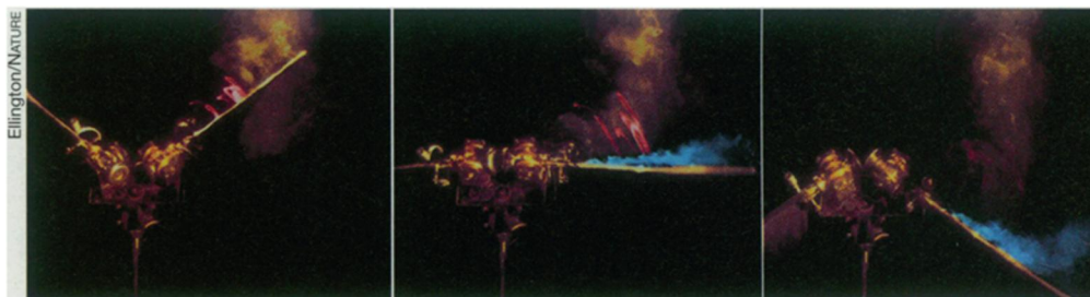
Inside a wind tunnel, the robotic hawkmoth injects blue smoke into the air flowing over its wings. The smoke, captured by vortices on the wing’s leading edge, widens during the downstroke (left to right). The robot avoids stall at the end of the downstroke, where the blue smoke begins to separate from the wing, by quickly beginning an upstroke.
