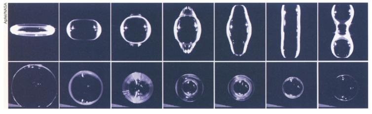
After being squeezed flat by sound waves, a drop of water enhanced with the surfactant Triton X-100 oscillates between a disk shape and a cigar shape (top sequence, side view) but maintains its symmetry (bottom sequence, top view) in an experiment aboard a 1995 mission of the space shuttle Columbia. The drop is 2.33 centimeters in diameter.
