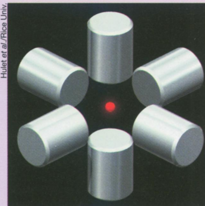
An array of six magnets traps a clump of lithium atoms chilled to a temperature near absolute zero.
