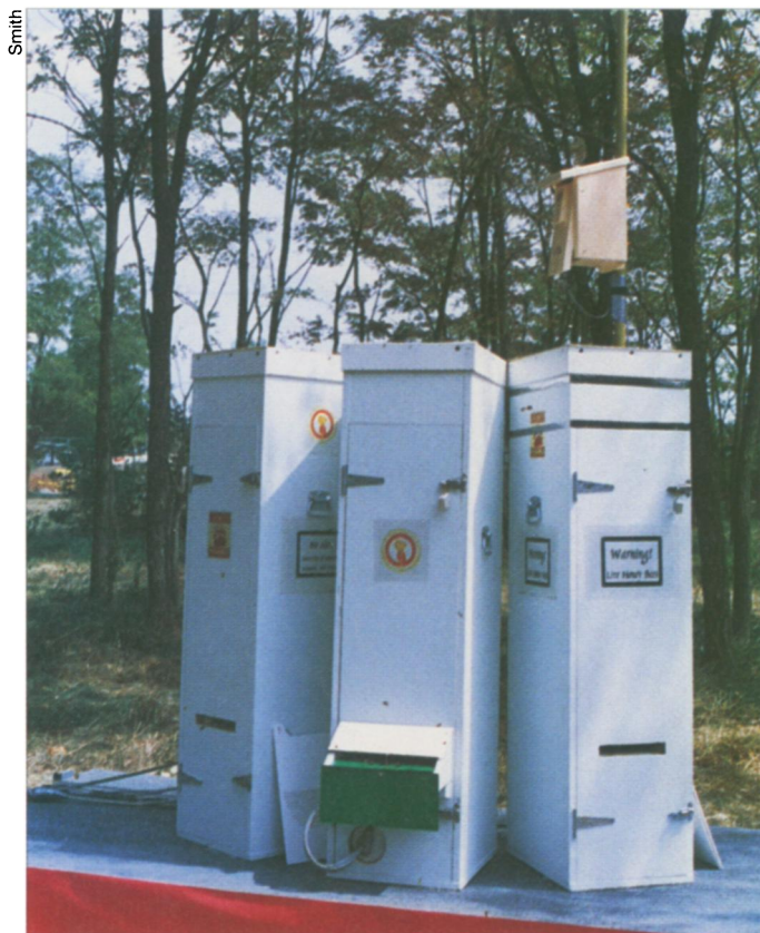
Three beehives outfitted with electronic sensors monitor a hazardous waste dump site in Maryland. A birdhouse on top conceals weather-monitoring equipment.
