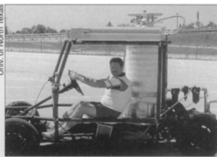
Engineer Mitty C. Plummer of the University of North Texas sits in a prototype vehicle powered by liquid nitrogen, contained in the insulated tank in the rear. The chassis and transmission come from a 1973 Volkswagen.
