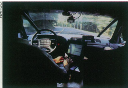
Self-guided cars allow their drivers to concentrate on other tasks, such as typing on a portable computer. A camera mounted on the windshield watches lane markings and controls the steering.
