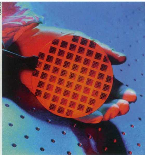
An array of integrated-circuit chips printed on a silicon wafer.
