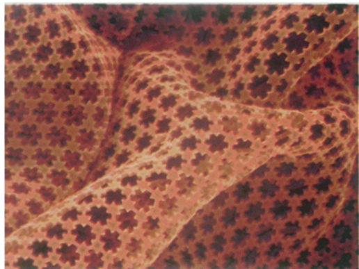
Plastic Microlace. Made of molded plastic, this fabric's narrowest links are about 1 micrometer wide. The original black-and-white scanning electron microscope image was digitally colored, and the colored version appeared on the cover of the Aug. 17, 1995 NATURE .
