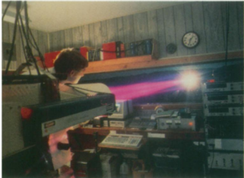
Researchers can gauge the warping of the land near the San Andreas fault using long laser beams.
