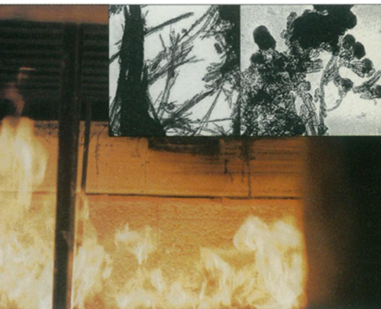
Asbestos treated with foam still protects building materials. With treatment, formerly carcinogenic fibers (left inset) become blobs of nontoxic minerals (right inset).
