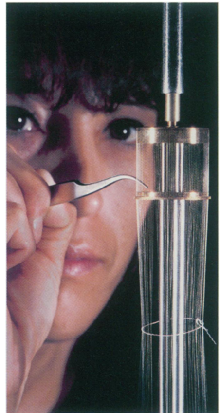
A cylindrical array of parallel wires—like the one shown as it is being fabricated—sits at the center of the Z machine.
