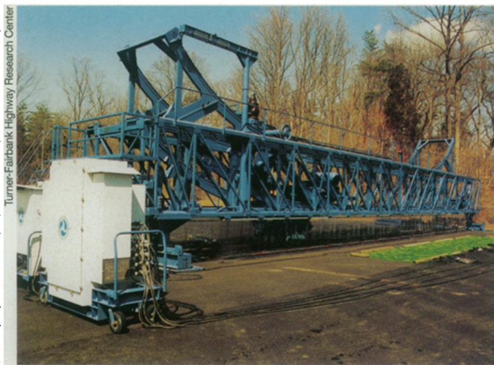
A machine called the Accelerated Loading Facility in McLean, Va., rolls a large truck wheel repeatedly across pavement to simulate traffic wear and tear.
