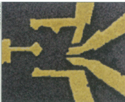
Scanning electron micrograph showing the surface of a quantum dot device, about 1 micrometer wide, made up of layers of gallium arsenide and aluminum gallium arsenide.
