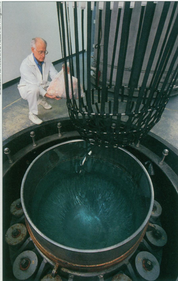
Bradford Berry about to load vacuum-packaged meat into a basket that will be placed into the water-filled Hydrodyning tank in Buena Vista, Va. The tank is then covered with a baffled dome, in background, to keep water from splashing into the air during the explosion and to muffle sound.
