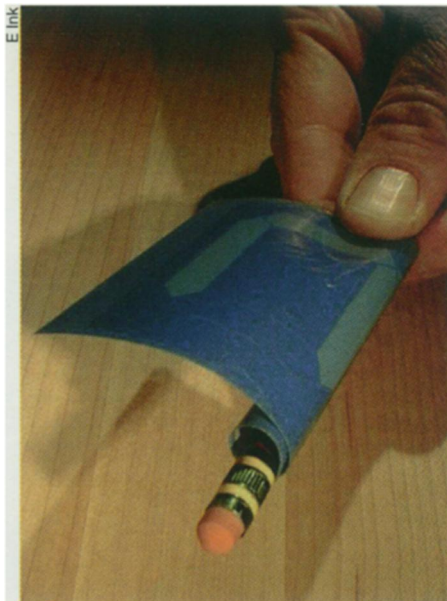
A high-contrast electronic-ink display has sufficient flexibility to be curled around a pencil.
