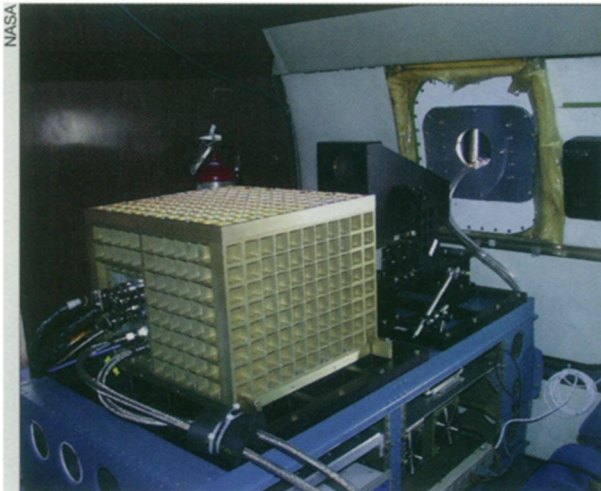
Flying over mountain ridges in Colorado, researchers are testing an experimental laser system designed to detect turbulence in clear air and provide advance warning.
