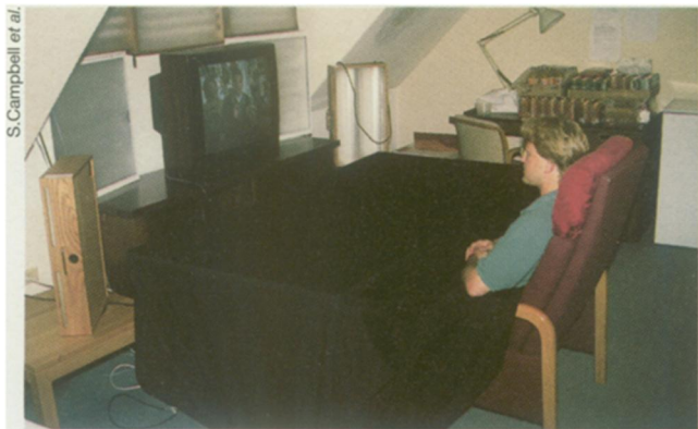
Volunteers sit at a table cloaked in black cloth to prevent outside light from reaching their knees.
