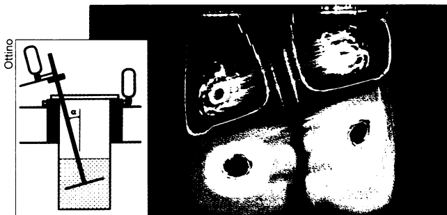
Fluorescent dyes illuminated by a sheet of laser light expose a vertical cross section of a liquid flow pattern in a mixing tank. Dark areas represent relatively quiescent regions of poor mixing, whereas stretched and folded dye streaks indicate chaotic regions of good mixing. Inset: A motor (yellow on left) rotates a tilted disk, which generates two rings of moving liquid, one above and one below the disk.
