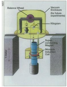
A kilogram weight on this sophisticated balance exerts a downward force that is countered exactly by the electromagnetic force generated when current flows in the movable coil in the superconducting magnet's field. By measuring the current, researchers link the upward force to ultraprecise constants that could be used to define an atomic-based kilogram.
