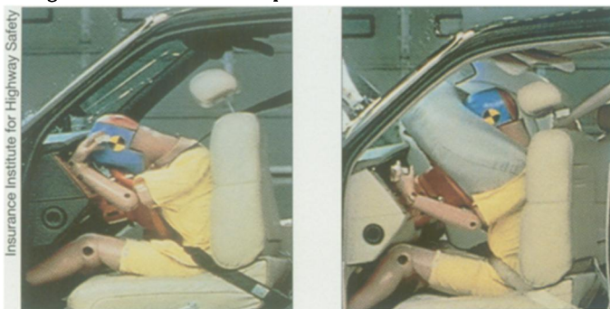
In most accidents, an air bag adds protection for the driver. In these crash tests at 35 miles per hour, a 5-foot-tall female dummy seated all the way forward suffers possible head, face, and neck injuries despite wearing a seat belt (left) but only possible neck harm in the air bag-equipped car (right).
