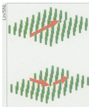
A missing row of posts in a photonic crystal (top) guides light straight through. When posts are removed to form a right-angle bend (bottom), almost all of the light also makes the turn.
