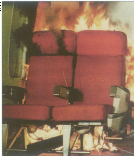
The Federal Aviation Administration sometimes tests the flammability of materials and equipment by building a mock airplane cabin and setting it on fire.
