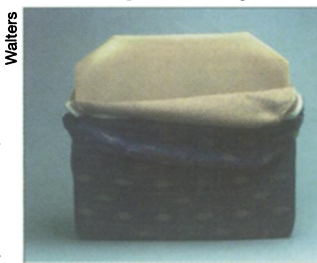
A layer of fireproof Kevlar encloses the flammable polyurethane in an airplane seat cushion.
