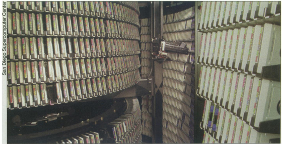
The San Diego Supercomputer Center hosts the world's largest data-storage system. This peek inside one of its three tape libraries reveals the robot arm (center) used to retrieve 10-gigabyte cartridges of filed data.
